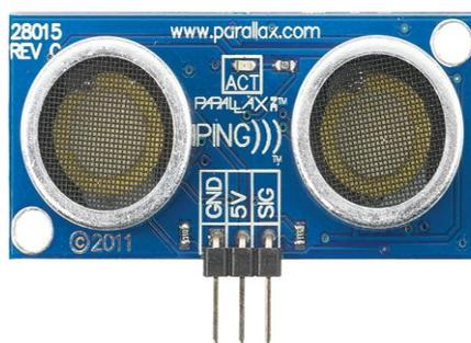
An ultrasonic sensor is an electronic device that measures the distance of a target object by emitting ultrasonic sound waves, and converts the reflected sound into an electrical signal. Ultrasonic waves travel faster than the speed of audible sound (i.e. the sound that humans can hear). Ultrasonic sensors have two main components: the transmitter (which emits the sound using piezoelectric crystals) and the receiver (which encounters the sound after it has travelled to and from the target).
