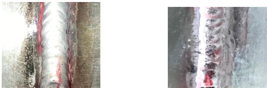
(a) Cracks on groove angle 45^\circ by ER4043 (b) Cracks on groove angle 60^\circ ER4043
