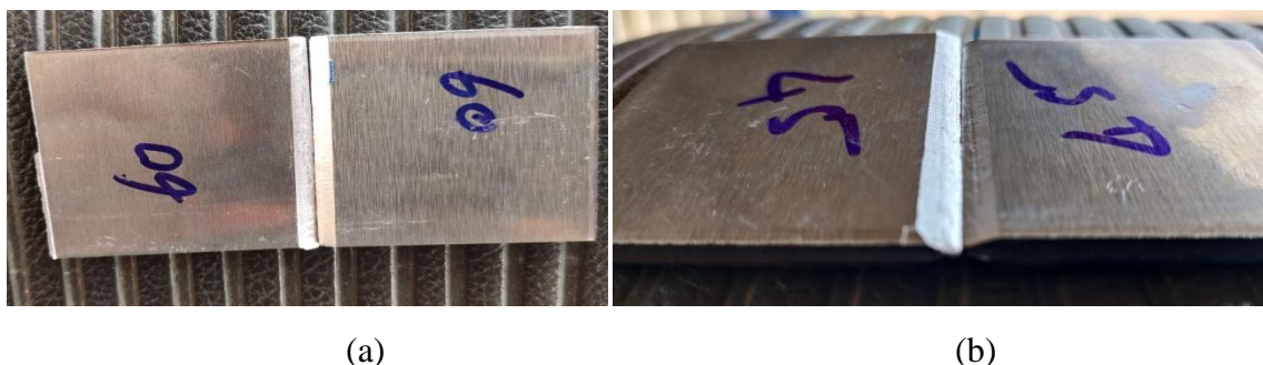
Fig 4. Double V groove on AA 6082 (a) 60° (b) 45°
