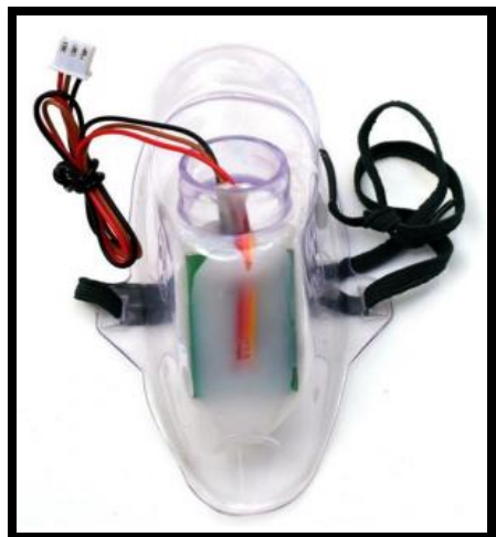
FIGURE 6: Respiratory sensor fitted inside a mask.
