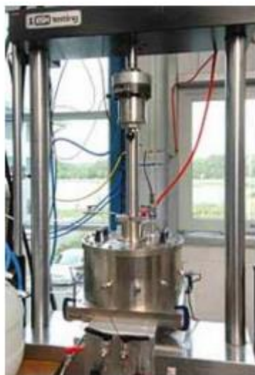
Figure:1 The corrosion-fatigue chamber Below figure shows a complex test chamber for CT-samples which we basically designed and completely tested. This chamber is mainly used for stress corrosion cracking tests of Aluminum and X-70 carbon steel CT-specimens
