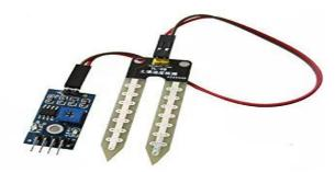
The dirt dampness sensor or the hygrometer is typically used to identify the mugginess of the dirt.
