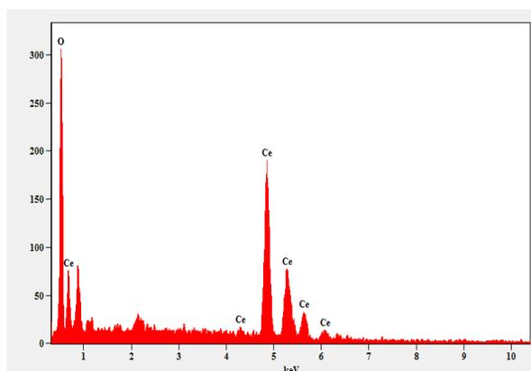
**Figure 4:** EDX of CeO<sub>2</sub> nanoparticles
