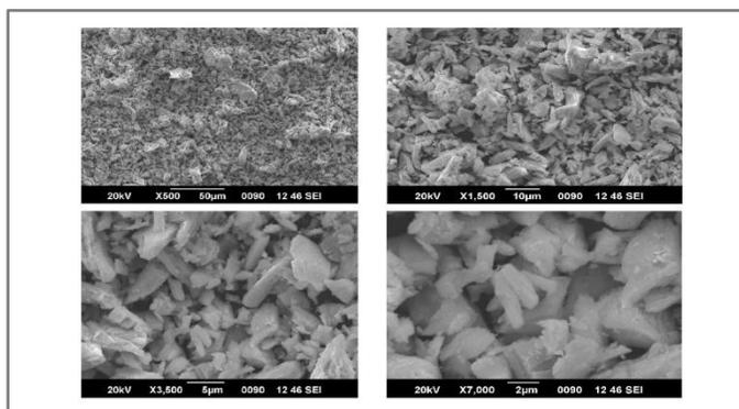
**Figure 3:**Scanning Electron micrographs of different CeO<sub>2</sub> nanoparticles
