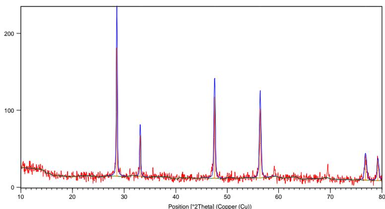
**Figure 5:** XRD Pattern of Synthesized CeO<sub>2</sub> NPs from *P.granatum* peel extract
