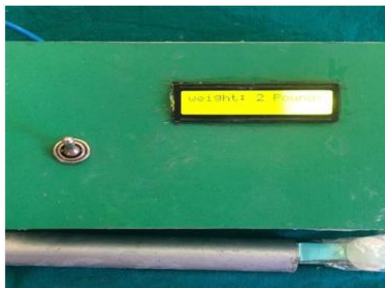
Figure 2 : Custom made occlusal force meter
