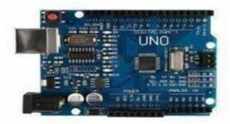
The suggested range of voltage is from 7 to 12 volts. It uses three types of memory. Code is
