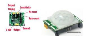
It detects whether the human is within the sensor's range or has moved out of the sensor's range. These are tiny, affordable, low-power, user-friendly and they have a wide range of the lenses. The Liquid Crystal Display module includes two rows. Each characterisassembledby a 5x8pixelbox. It isoperated on two modes. It works faster on 8- bit mode than 4- bit mode. The operating voltage varies from 4.7 to 5.3V and the current utilization is 1 mA.
