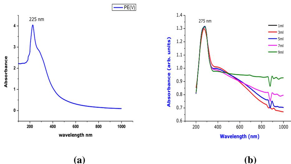
**Figure 2. UV-visible spectral study of (a) plant extract of *Allium fistulosum*, (b) plant extract with PdNPs.**
