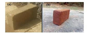
The clay brick contains the materials of clay, egg shell powder. The adopted mix ratio is 1:4. By adding these materials the proportional quantities be will assigned. The size of the brick is 9x4x3 inches.
