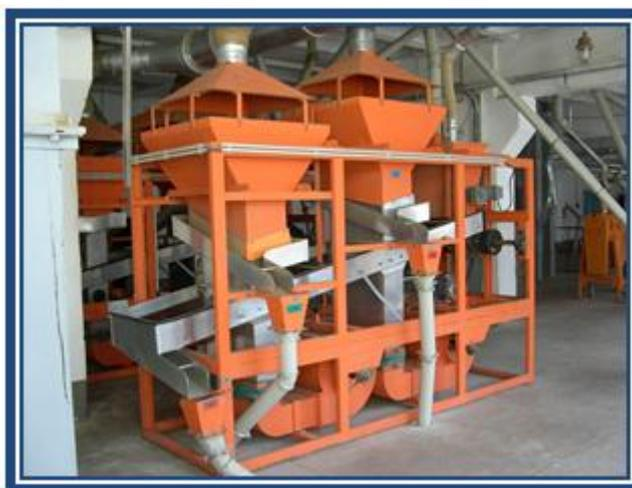
**Fig. 3. Aspiration column for sorting seeds by aerodynamic properties**
