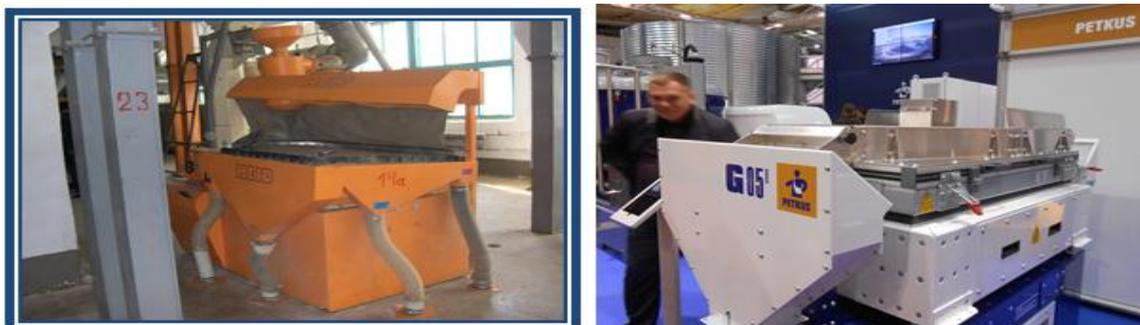
**Fig. 6. Pneumatic sorting tables for sorting seeds by specific mass**
