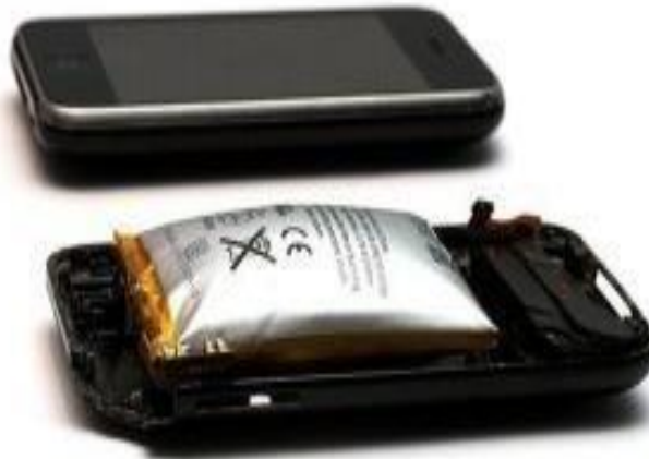
Figure 1. Issue caused due to overcharging of battery
