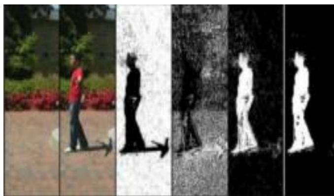
Fig.6. Detection of human from background subtraction
