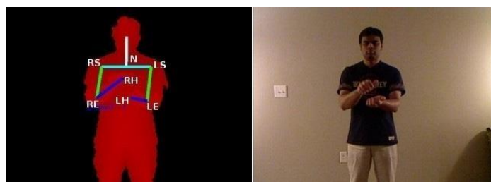
Figure 2. Features extracted (left) from gesture described by participant (right) built from Kinect 3D depth image (Fig. 6.[7])
