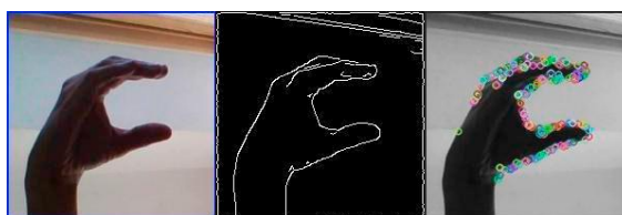
Figure 6. From left to right – original image, segmented edge image using Canny edge detection, ORB features. (Fig. 3, 4, 5 [18])
