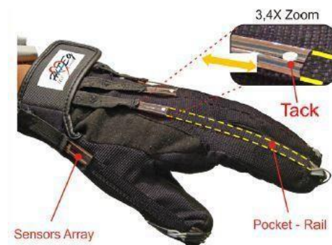
Figure 3. A goniometric glove with sensor array containing flex sensors to give the measure of bends in finger and wrist. (Fig.4. [11])
