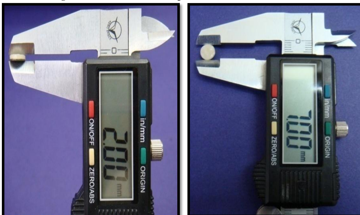
Figure 5 Dimensions of The Specimen (Thickness & Diameter)
