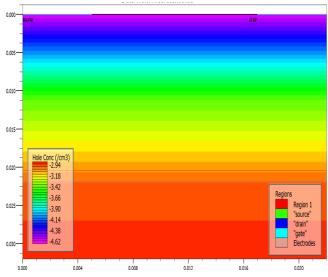
This refers to the "free" electrons and holes. They carry charges (electron -ve and hole +ve), and ar chargeable for electrical current
