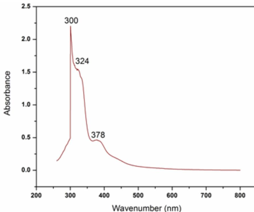
**Fig.3: UV-Vis Spectrum of 4PMN molecule**
