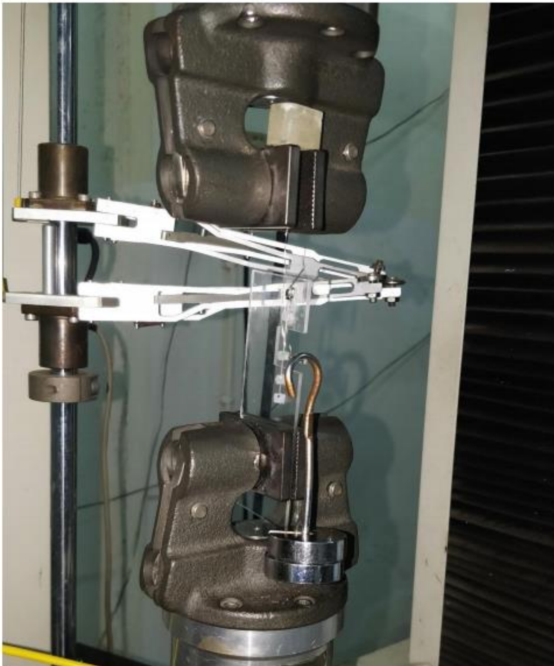
Figure 8 - FRICTION TESTING USING UNIVERSAL TESTING MACHINE
