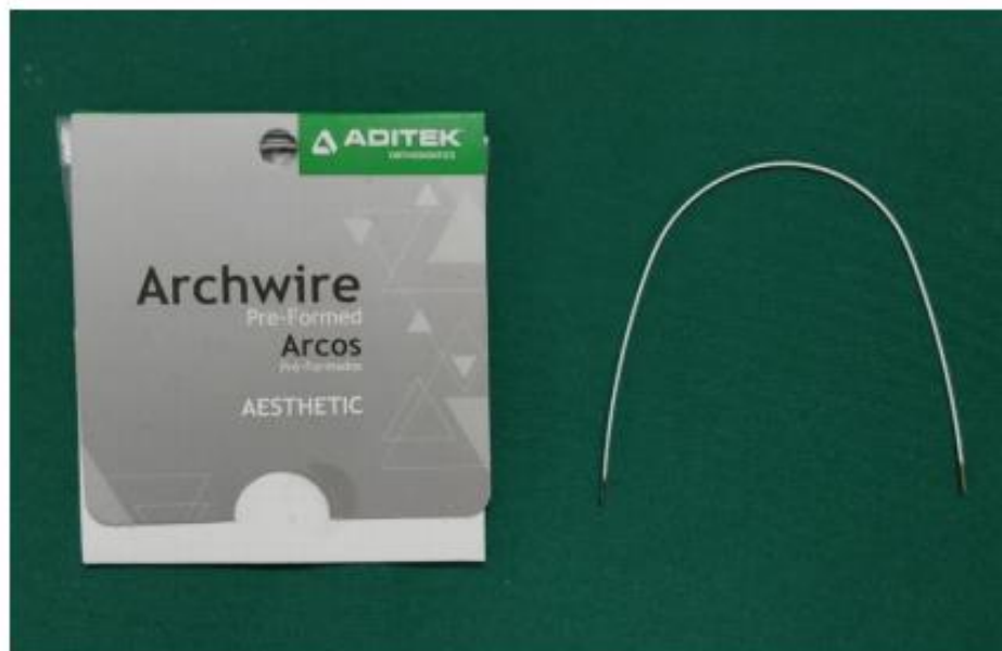
Figure 6 - GROUP III SAMPLES- TEFLON COATED WIRES (ADITEK)
