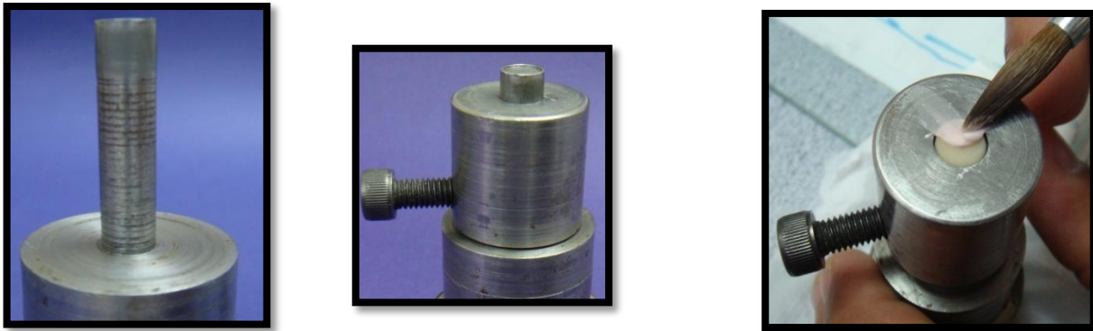
Figure 4 Specially Fabricated Stainless-Steel Die (II) For Veneering
