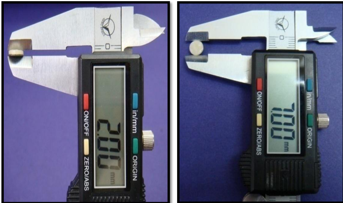
Figure 5 Dimensions of The Specimen (Thickness & Diameter)
