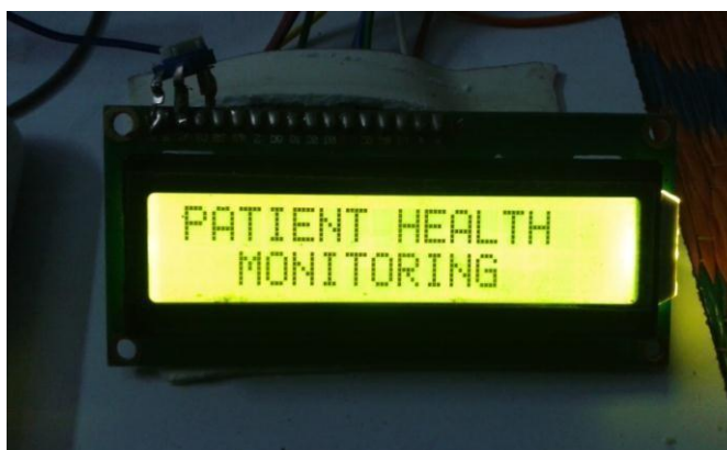
Fig. 11 LCD display showing the initial message
