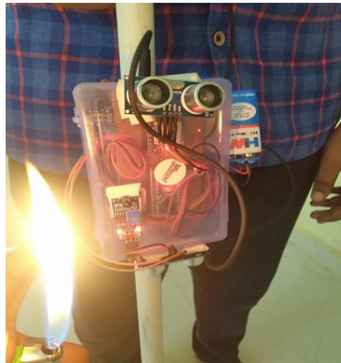
Figure 8. Device detecting the flame and alerting the user
