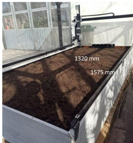
Figure 4: FarmBot's field dimensions
