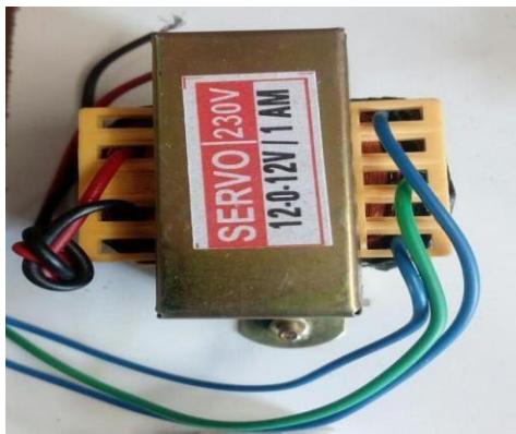
Figure 7:STEP DOWN TRANSFORMER
