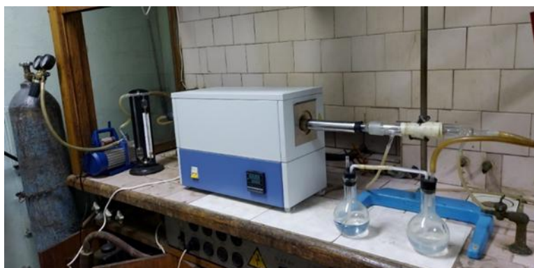
Figure 5. Laboratory installation for the sublimation of silicon and titanium fluorides
