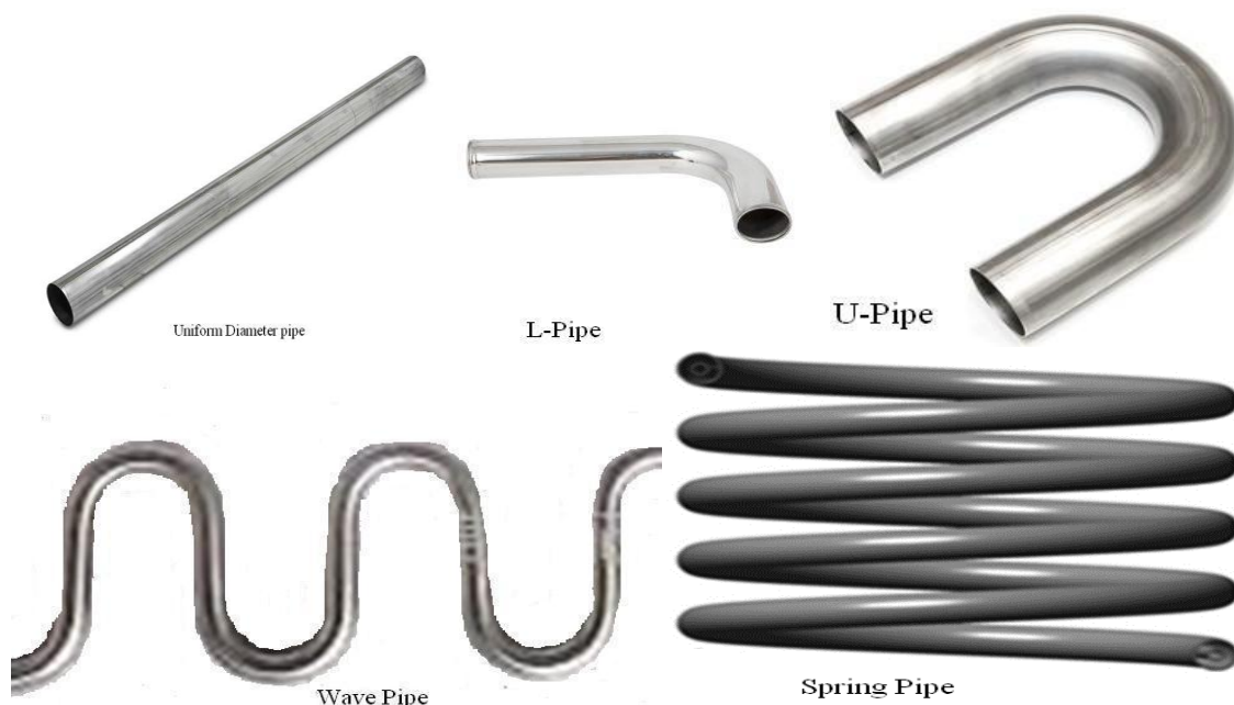
Figure 1: Different geometrical models for analyse the heat transfer in multi-phase flow.
