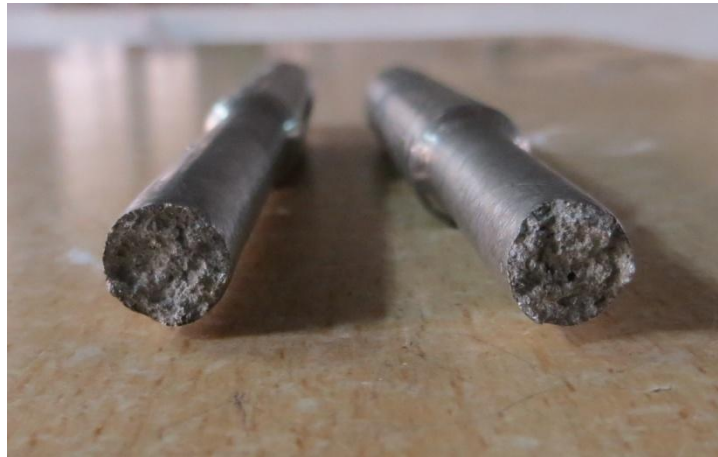
Fig 2.1 Specimen after the Tension Test
