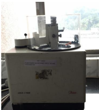
Figure 6: Hard Tissue Microtome -LEICA-SP-1600
