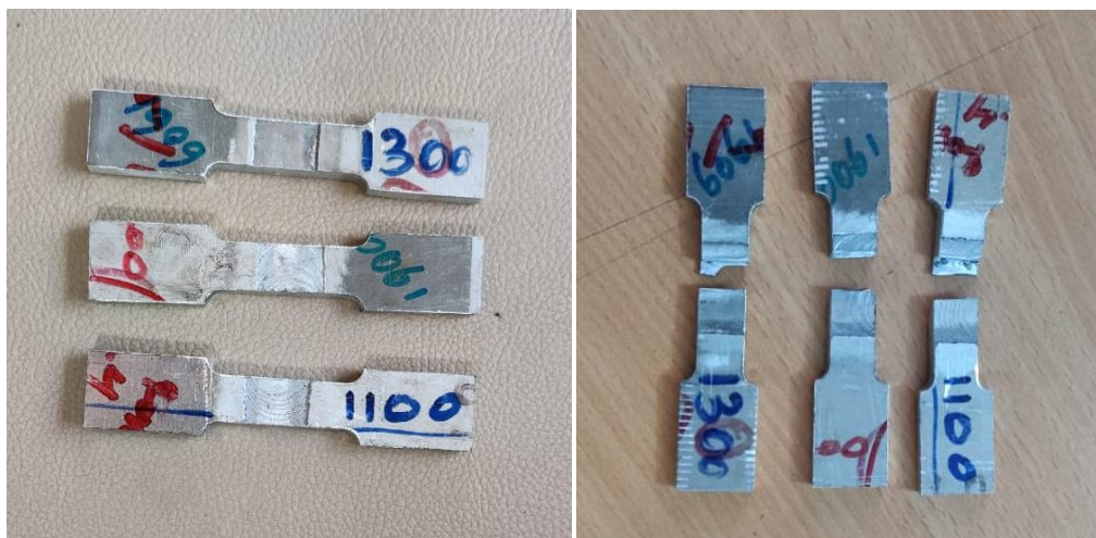
Figure 3. Test specimens before tensile test Figure 4. Test specimens after tensile test
