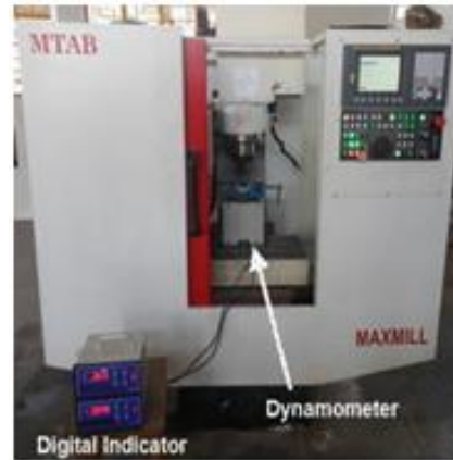
Figure 1. CNC Drilling machine Experimental Set up
