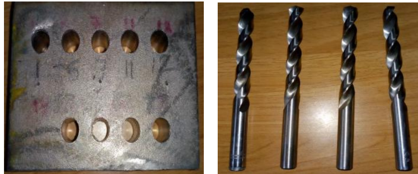
Figure 2(a). Workpiece for completed Process Figure 2(b). HSS Drill tool
