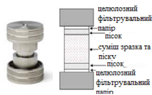
Figure 2. Stainless steel cells with a volume of 1 ml and the schematic diagram of a packaged extraction cell with layers of cellulose filter paper, sand and a mixture of sample and sand.
