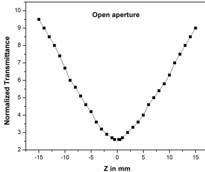
Figure 8 Z-scan pattern for the sample in open aperture
