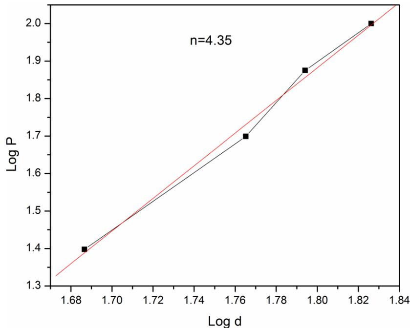
**Figure 6 Plot of log P versus log d of TGSSu crystal**
