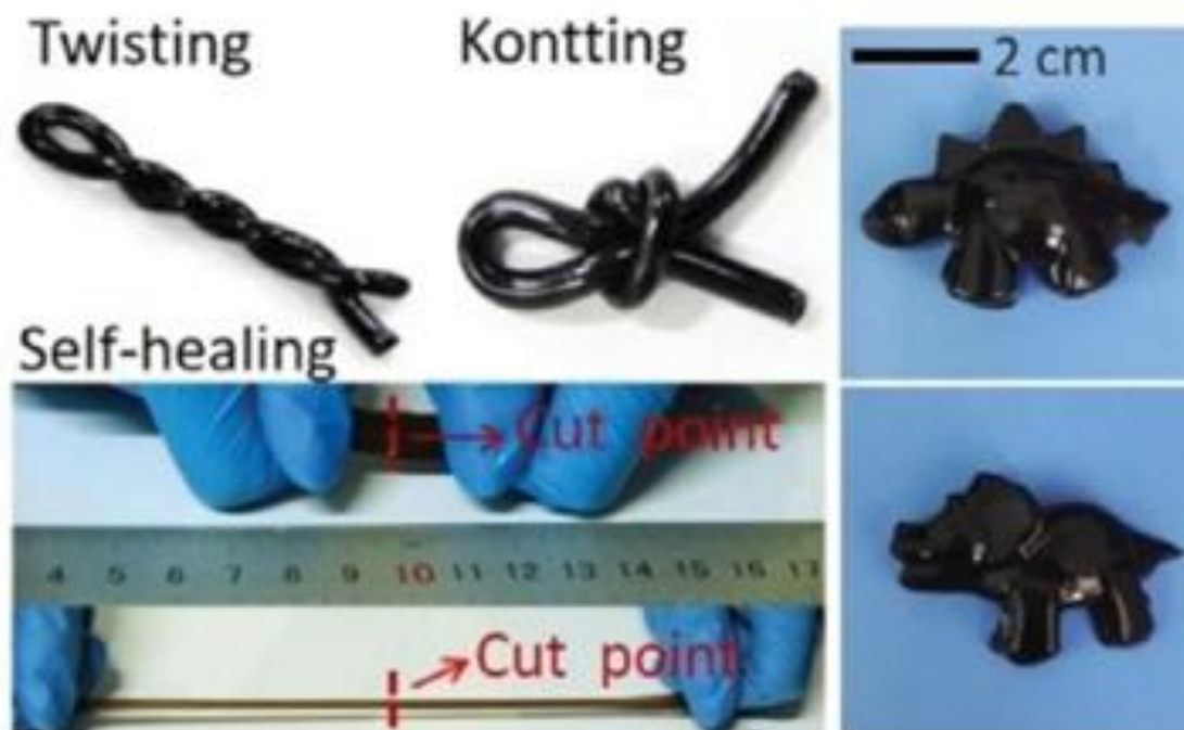
Figure 4: Stretchable, self-mending, and glue particle gel nanocomposites for strain detecting.[33][34]
