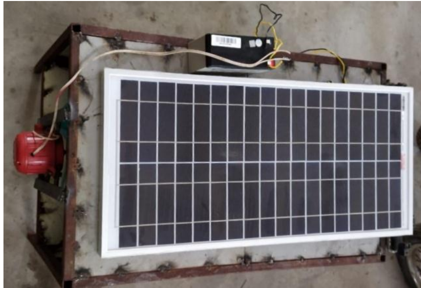
Fig.2 Experimental Setup of solar air conditioner using peltier module
