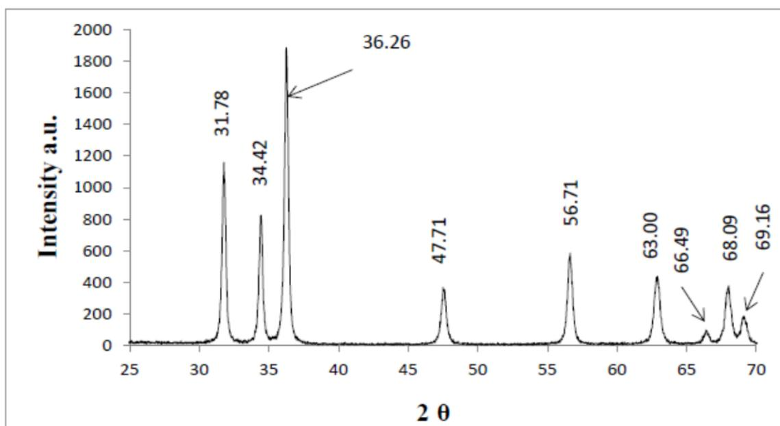
**Figure 1.** XRD patterns of zinc oxide nanoparticles
