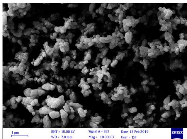
**Figure 6.** Scanning electron microscope images of copper oxide nanoparticles
