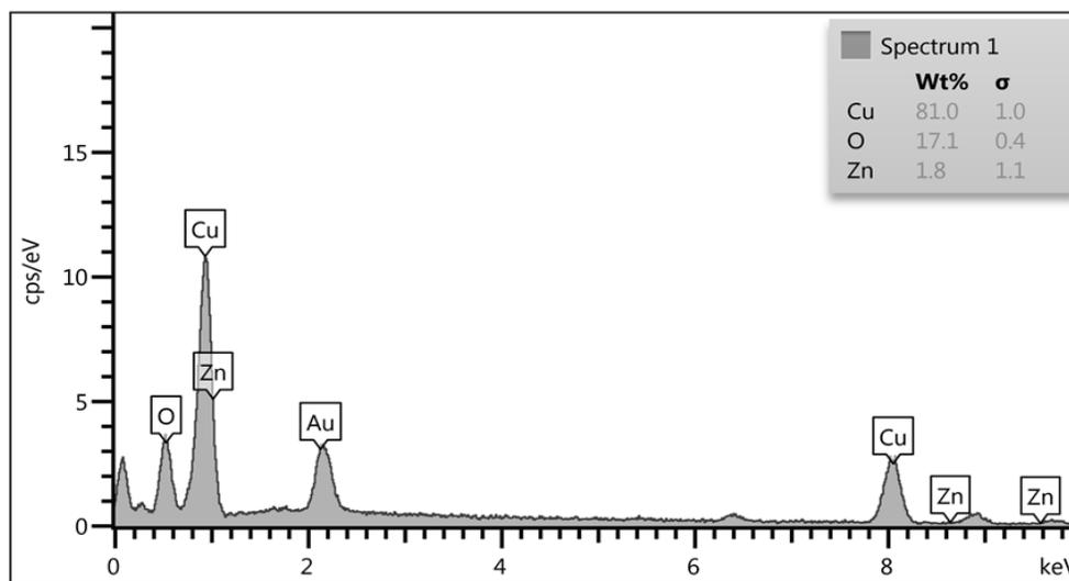
Figure 4. EDX curve for copper oxide nanoparticles
