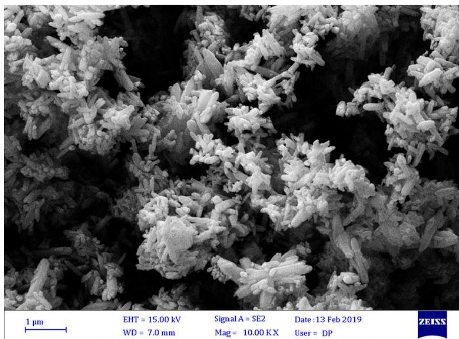
**Figure 5.** Scanning electron microscope images of Zinc Oxide nanoparticles
