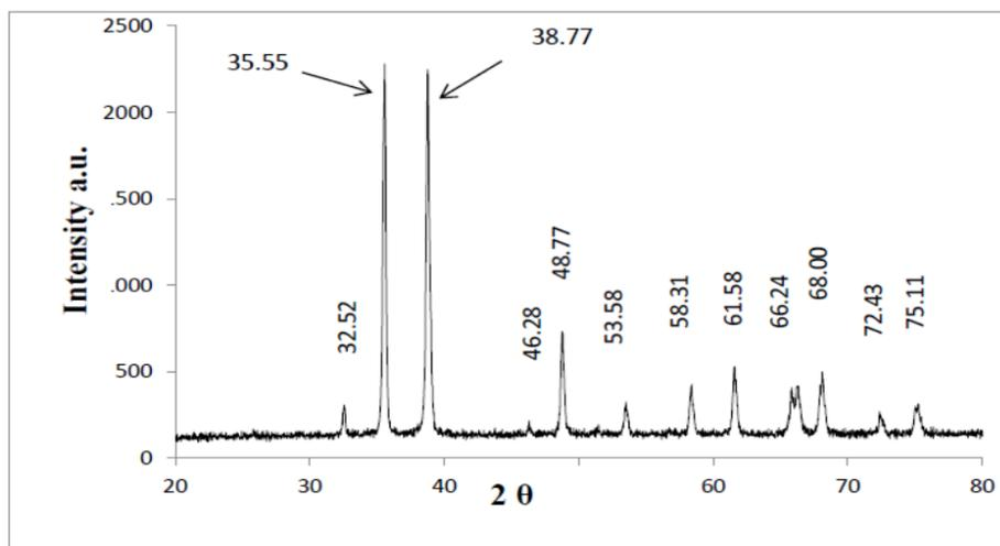
**Figure 2.** XRD patterns of copper oxide nanoparticles
