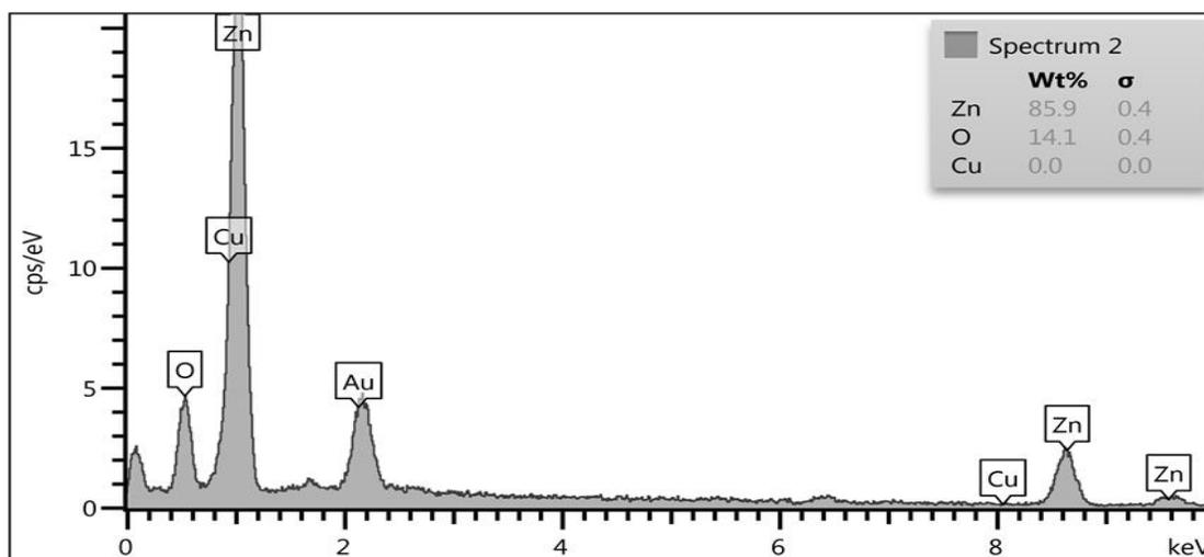
Figure 3. EDX curve for nanostructured zinc oxide
