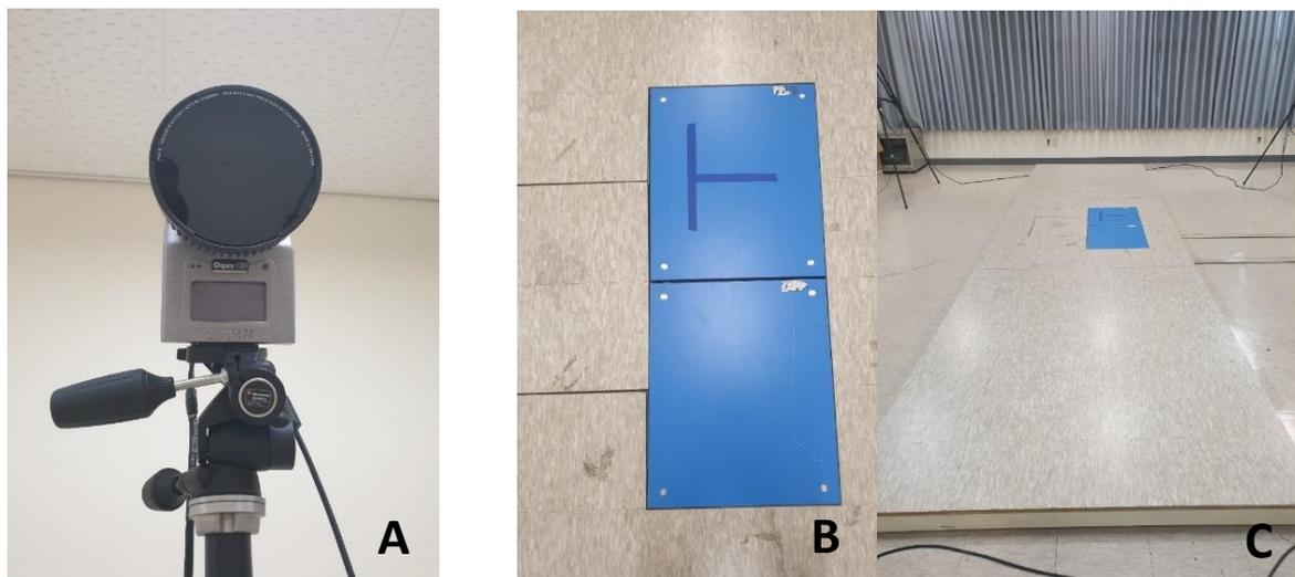
Figure 3. A:Qualisys system-Qualisys Medical AB4113, Gothenburg, Sweden, B:Force plate, C: 6m walk way
