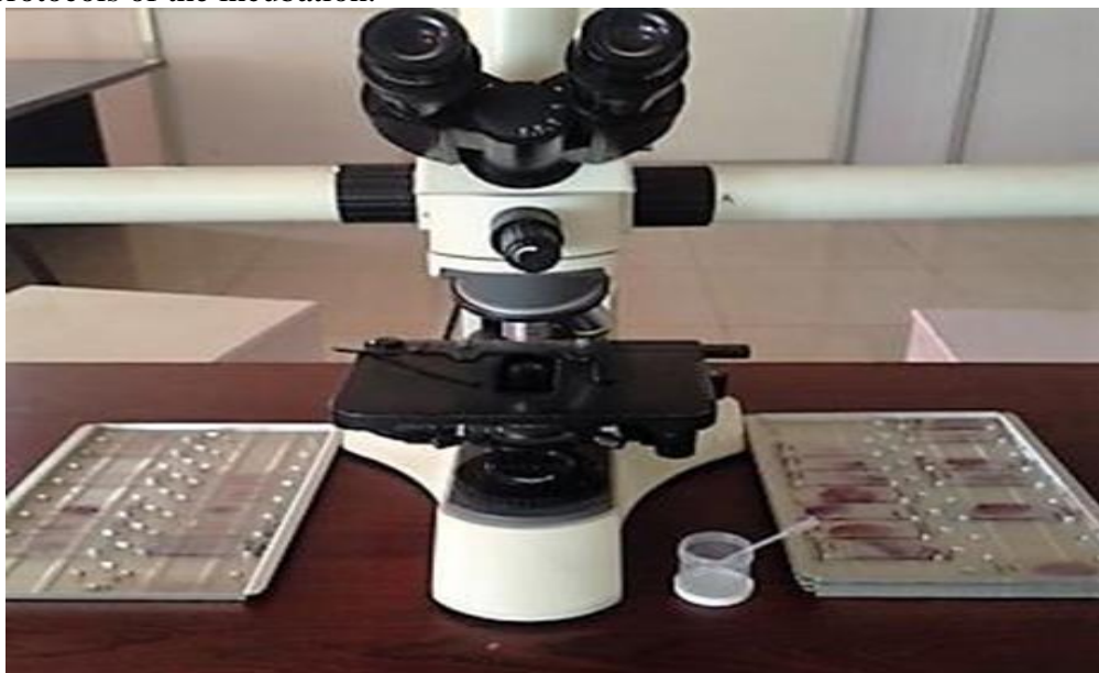
Figure 5 Microscope (multiviewing microscope) CXR 5; AC 110 V, 60 Hz. 60 V A, T250V, 500mA
