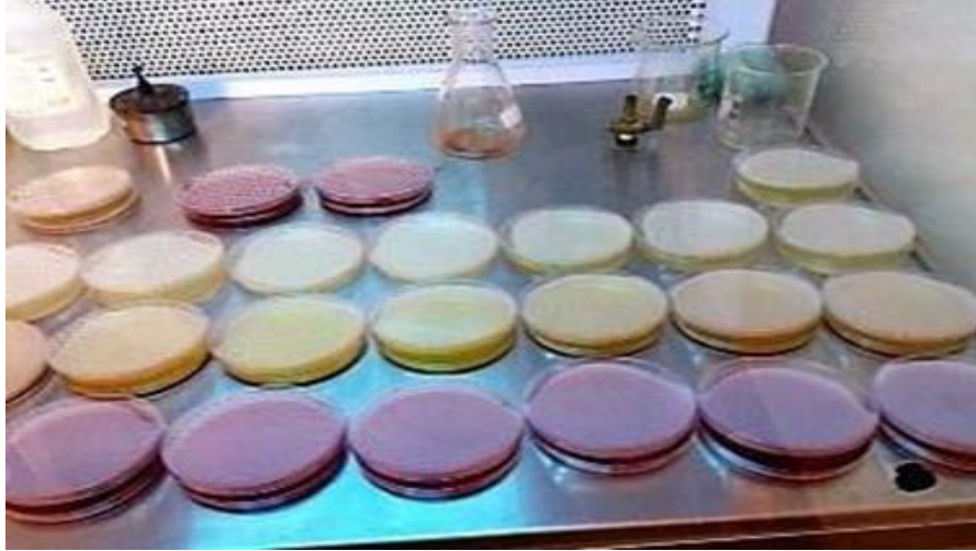
Figure 4: Laminar Flow Chamber with Culture Dishes
