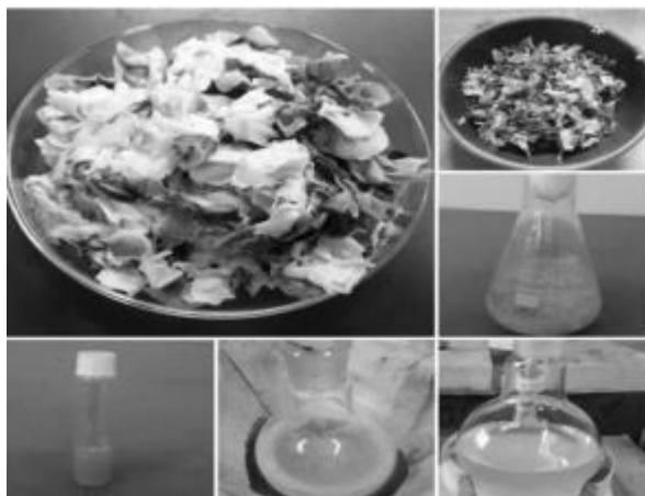
Fig 2: Steps for Oil collection from Fish Skin
