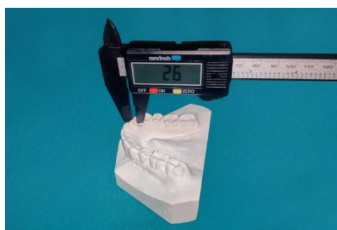
Figure 1: Vernier caliper used to assess crowding in dental cast
