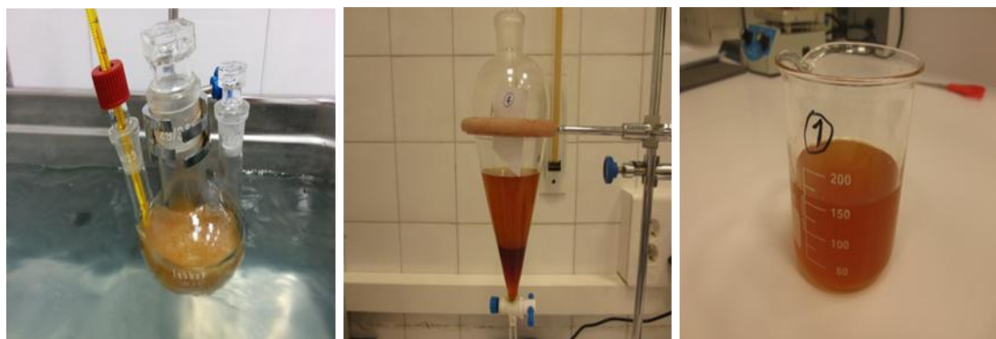
Figure 1: Reactor detail, reaction reaction decanting and Detail of stored biodiesel sample
