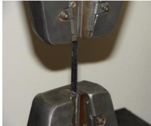
Fig 6.3(b) Specimen fixed in Jaws
