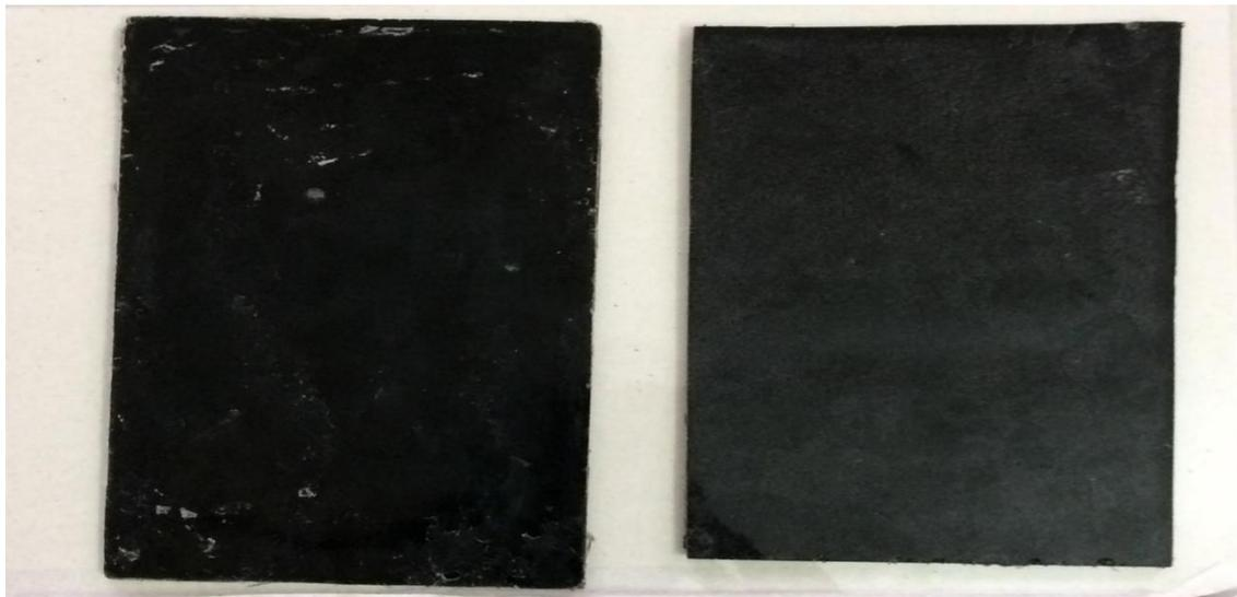
Fig6.8(b):Epoxy+Coconut Shell Ash composite and Epoxy+Rice Husk Ash composite.
