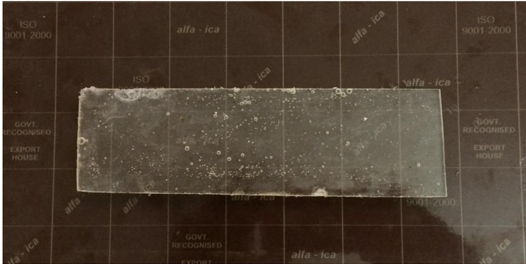
Fig6.8(a):Epoxy sheet(without fiber and filler)
