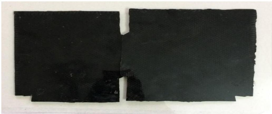
Fig 6.8(d): Epoxy +Carbonfiber+RiceHuskAsh composite(70:25:5),Epoxy+Carbonfiber+RiceHuskAshcomposite(65:25:10),
