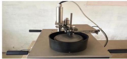
Fig6.5(a) Pin on Disk wear testing machine Fig6.5(b) Specimen fixed in Arm
