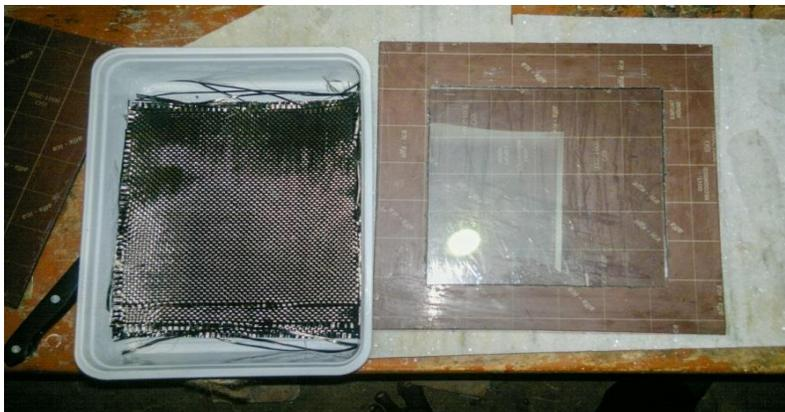
Fig5.2–Carbon fiber mats and mould
