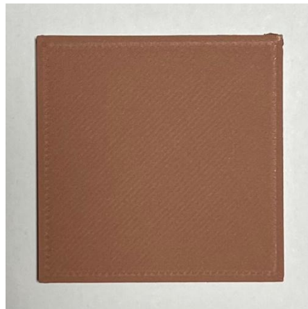
Fig. 4. Radiation shielding. Shielding made by varying nozzle size and layer height as each filament is printed.
