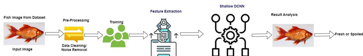
Figure 3: Deep CNN (Feature Extraction) and Classification
